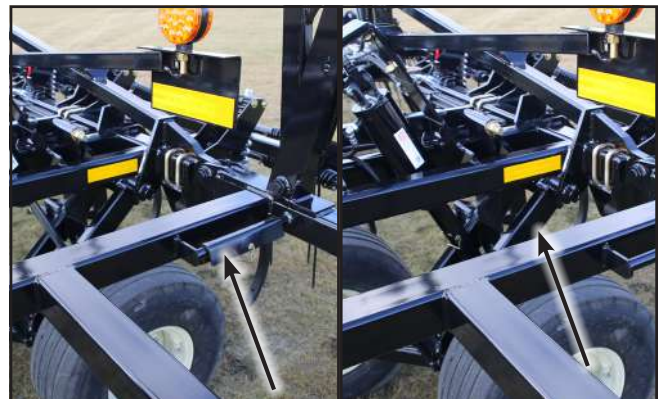
Fig. 45 Cylinder Stop: Removed and Stored/Installed
