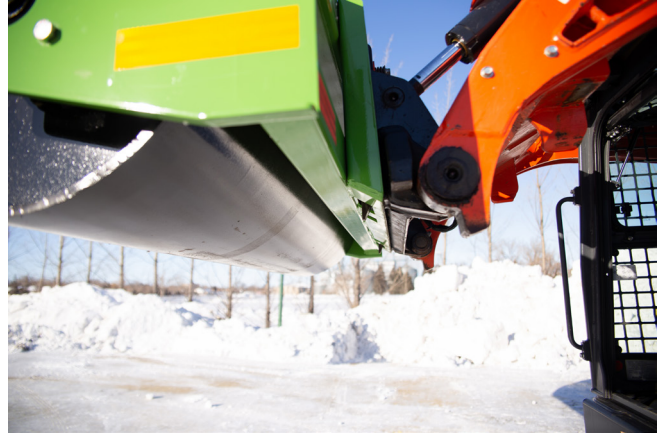
Fig. 5 Lower lock pins engaged.
