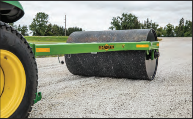
Fig. 51 Wash Machine: Single Land Roller
