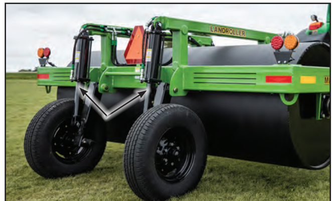
Fig. 35 Cylinder Stops Installed
