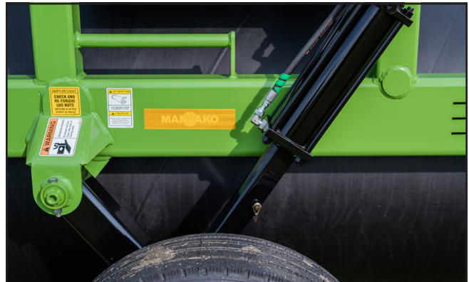
Fig. 37 Cylinder Stop installed
