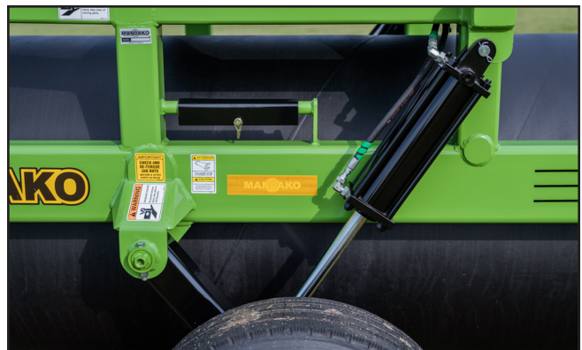
Fig. 38 Cylinder Stop removed and stored
