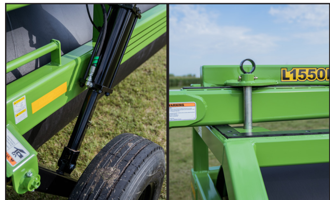
Fig. 45 Ensure Cylinder Stops and Frame Lock Pin are in place and secure
